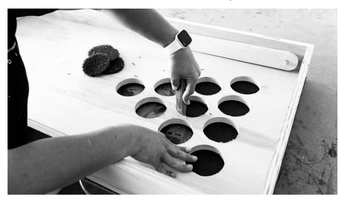
Once the astro turf is attached, flip the game board over and cut out the holes with a sharp razor knife.
