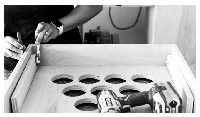
Use a 3/4" piece of wood as a block at the front edge of the game board frame. Place the leg against that block to set the location for the legs. Drill a 3/8" hole through each leg and through the side of the game board frame. Attach the legs with 2 1/2" carriage bolts and locking nuts, tightening them enough to hold the legs in position, but still allow for them to be folded back down into place when not in use.
