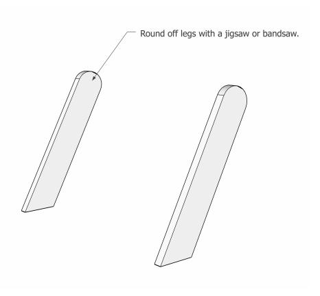
Use a small cup to mark the tops of the legs where they will be rounded off. Using a jigsaw or a bandsaw, round off the tops of the legs to allow them to turn into position and fold up when the game is not in use.
