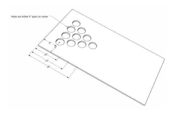
Mark the locations for the holes on each game piece. For the first row, measure down 6". Use a square to mark a line across the board. The first hole is 6" in on center from the side of the board. The remaining holes are 4" apart on center.
