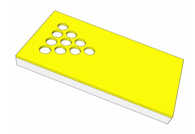
Drill 1/16" pilot holes around all four edges of the top. Add a bead of wood glue to the top of the frame, then center the top onto the frame. Attach with 1 1/4" wood screws.
