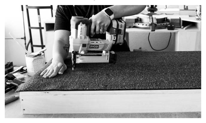
Cut the astro turf to size using a sharp razor knife. Apply a generous coat of contact cement onto the top of the game board with a paint brush. Align the grass over the game board and begin stapling it to the top starting at one edge and working your way down, smoothing out the grass as you go.
