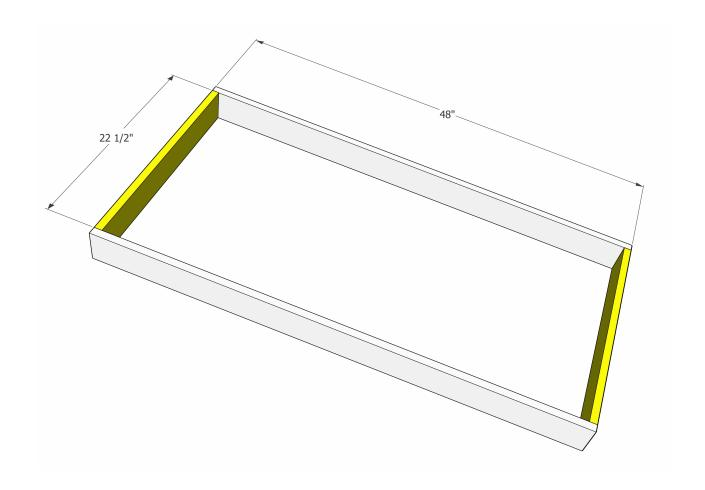
To build the frame, drill two 1/16" pilot holes into each end of the 48" boards. Glue and clamp the frame together, then attach the pieces with 1 1/4" wood screws.
