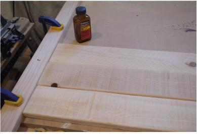
3. CUT (2) lengths of your 1" x 2" cedar board to the same width as the three boards you just glued together. Sand and then screw to your glued boards using #8 1 1/4" screws.
